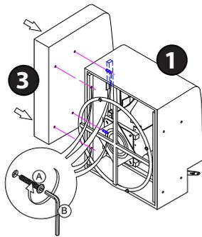
1. Tip the seat base 1 on its back side as shown. Align the holes of left arm 3 with holes in left side of seat base 1. Insert Bolt A into hole in 1 and affix to 3. Use allen key B (included) to tighten.
