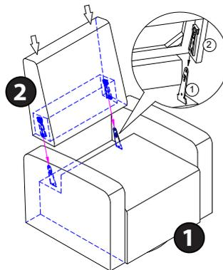
5. Select 1 - Seat Base and 2 - Back Rest. With Back Rest Buttons facing inward, carefully align backrest mounts to seat-base mounts. Insert bottom backrest mounts into Seat Base Mounts until they latch and backrest is secured to seat-base. Exercising Caution, Carefully lift upward on the backrest to confirm backrest is secured.
