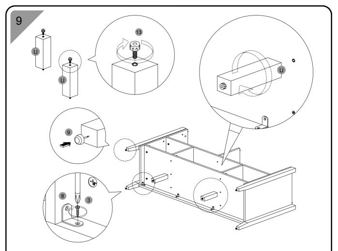
• Install Screw Stud (13) to leg (U) before assembling them to bottom panel (G) as shown. Attach Plastic Feet (10) & L Bracket (8) with screw (3) as shown above.
