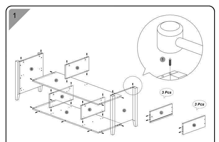
• Install 39pcs of Wooden Pins (1) into all panels as shown. Use a wooden hammer or light rubber hammer to avoid damage to the pins. Please pay close attention to which holes you have to use, and do not join any parts yet!
